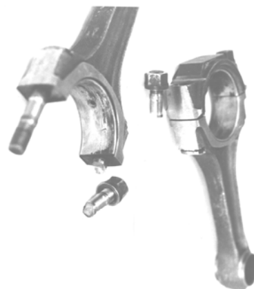
Fig1. The nature of the destruction of the connecting rod bolt due to the weakening of the tightening force
