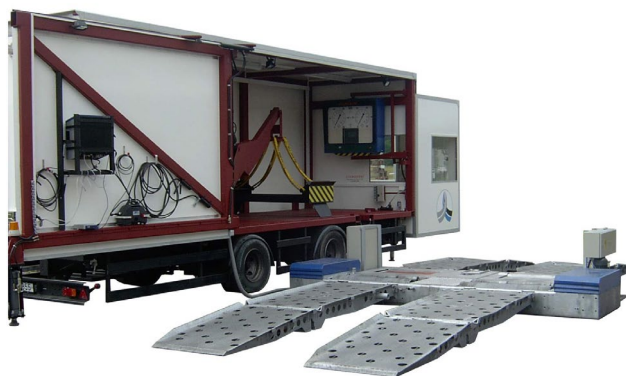
Fig. 3. Comprehensive roadside inspection station Energotest MVA-40 (Hungary)
