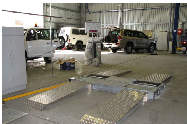
Fig. 7. Mobile braking roller stand BM3010 (Denmark)
