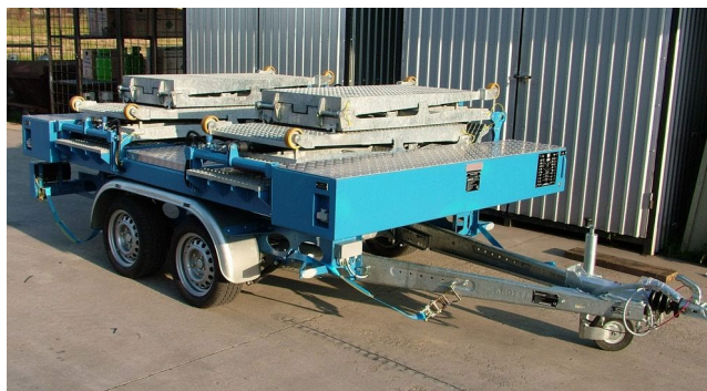
Fig. 2. Mobile technical control station Energotest BRZ-20 (Hungary)
