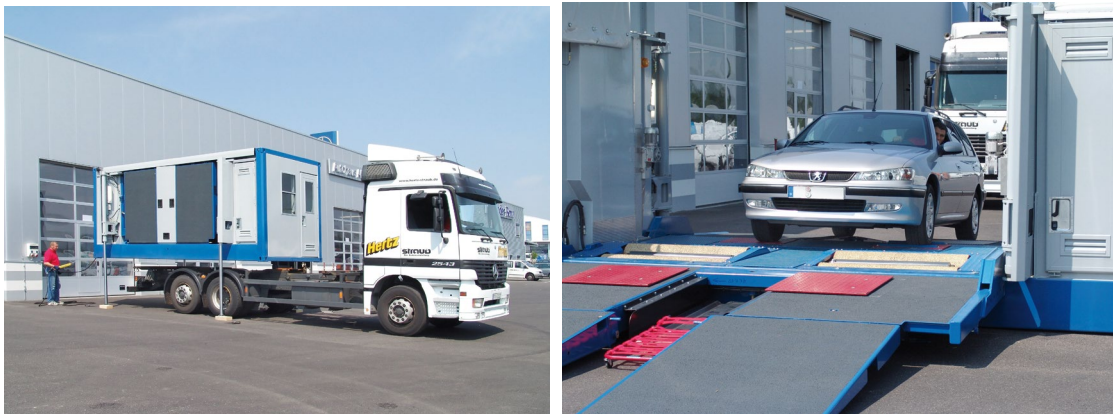
Fig. 5. Universal mobile station for technical control of all types of motor vehicles MTL-15 by MAHA
